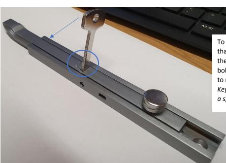
To unlock the bolt, you'll need the key that is provided with the bolt .Place the key into the hole on the face of the bolt and then push the key to the side to move the lock tab of the bolt. The Key has to be pushed to the side as it is a spring loaded mechanism
