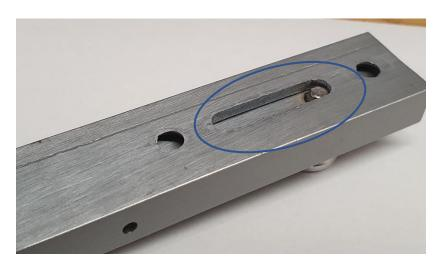
When the bolt has been put back together you need to screw the knob/screw back in and make sure that the end of the screw is in the slot as shown
