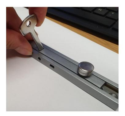
Whilst you have the key pushed to the side you will need to pull the bolt down the case to have the bolt in the open and unlocked position
